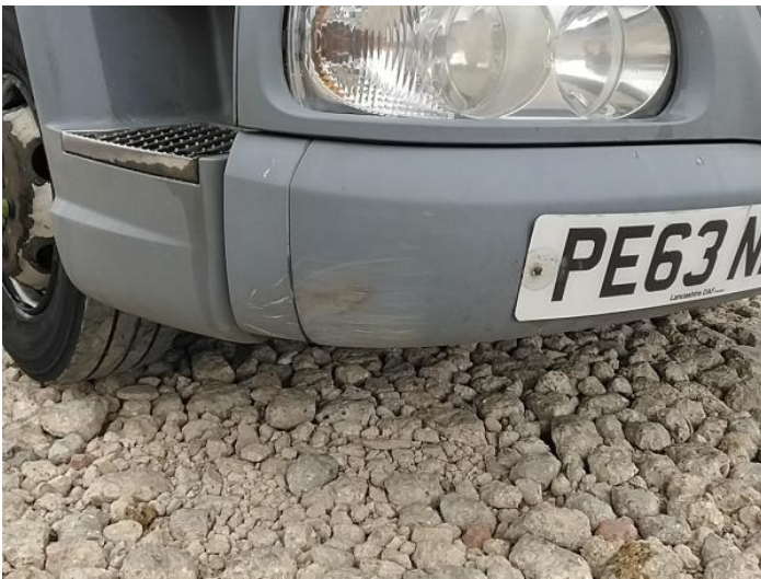
5: Bumper Front Moulding Scuffed (Unpainted) UpTo 100mm
