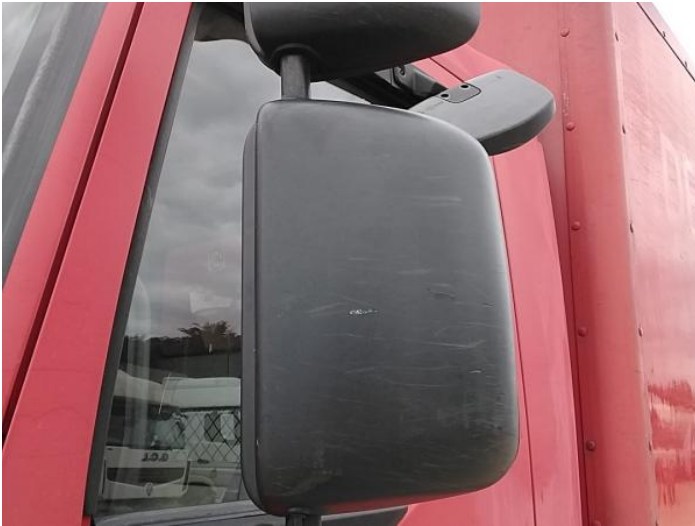
9: Door Mirror Assy nsf Scuffed (Unpainted) UpTo 100mm
