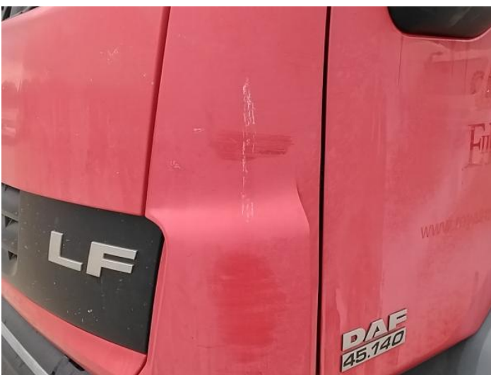
7: Wing nsf Scratched UpTo 25mm Not Thru Paint
