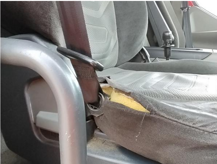
17: Seat Base Cover osf Holed Over 3mm
