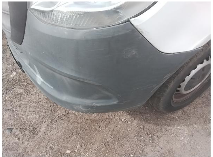
2: Bumper Front Scratched Over 100mm Thru Paint
