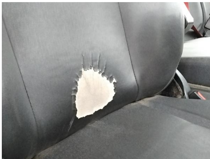
10: Seat Back Cover osf Torn Over 3mm
