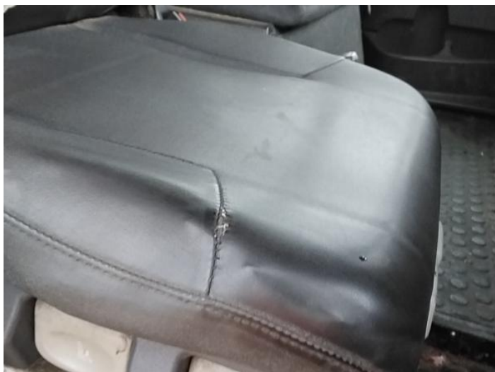
9: Seat Base Cover osf Torn Over 3mm
